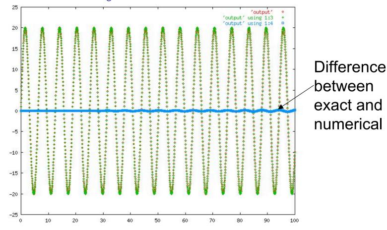
gnuplot> set term jpeg Terminal type set to 'jpeg' Options are 'small size 640,480 ' gnuplot> set output 'displace.jpg' gnuplot> plot 'output','output' using 1:3,'output' using 1:4
