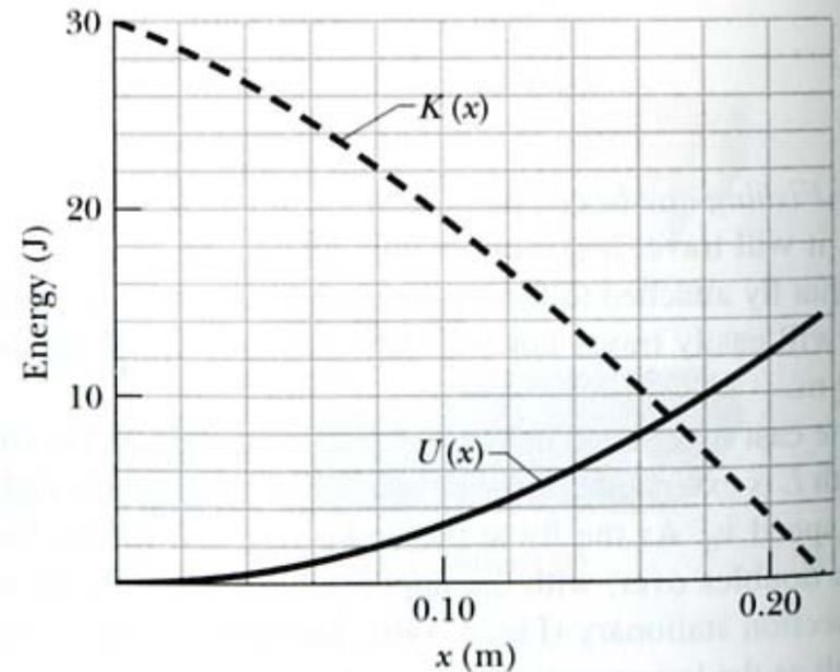
**B1.** A 2kg block is pushed against a spring with spring constant  $k=500$  N/m compressing it 20 cm. After the block is released, it travels along a frictionless horizontal surface and a  $45^\circ$  incline plane. What is the maximum height reached by this block?
