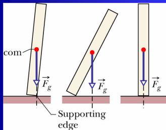
(1) Torque about supporting edge by  $F_g$  is 0 because line of action of  $F_g$  passes through rotation axis → domino in equilibrium.
