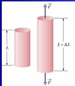
**Tensile stress:** associated with stretching
