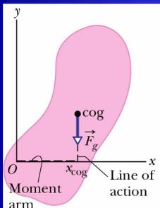
$$x_{cog} \sum_i F_{gi} = \sum_i x_i F_{gi} \rightarrow x_{cog} \sum_i m_i g_i = \sum_i x_i m_i g_i \rightarrow x_{cog} \sum_i m_i = \sum_i x_i m_i$$
