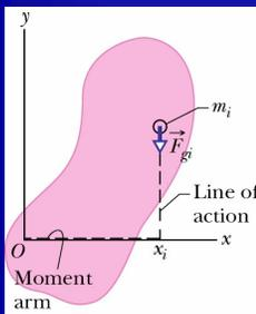
Each force  $F_{gi}$  produces a torque  $\tau_i$  on the element of mass about the origin O, with moment arm  $x_i$ .
