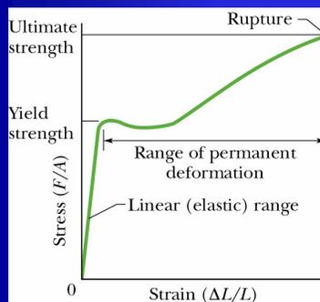
(1) Stress = cte x Strain → Recovers original dimensions when stress removed.
