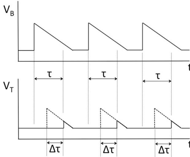
Fig. 2. Clocking and sensing waveforms. A periodic ramp voltage is applied to each pixel at the frame rate. Electrostatic repulsion breaks the tip contact, so that  $V_T$  is initially zero. As  $V_B$  decreases, the tip re-contacts after a time  $\tau$ , when the remainder of the waveform appears at  $V_T$ . Downward deflection of the thermal bimorph shortens  $\tau$  by  $\Delta\tau$ , which is a measure of the amount of absorbed heat.
