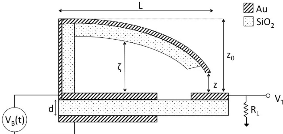
Fig. 1. Schematic of clocking cantilever heat sensor. A periodic saw-tooth bias  $V_B$  is applied between a buried electrical plate and a surface plate which is electrically connected to the flexible bimorph cantilever, which is comprised of gold and oxide. When the tip contacts the tip pad, the bias voltage appears at the output  $V_T$ .
