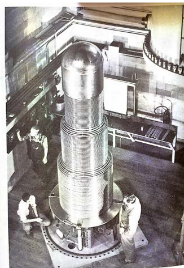
PLATE IV. Large (5-MeV) Van de Graaff generator is shown here with its pressure cover (upper right) removed. Note the polish of the high-voltage terminal at top. Rings around the column are voltage dividers. In this M.I.T. installation the laboratory for experiments with beams is below the machine.
