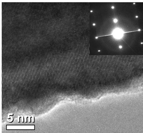
Fig. 3. The high-resolution TEM images and the inset with the selected-area diffraction pattern of the single-crystalline ZnO nanorods grown by self-assembly method.
