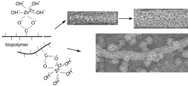
Fig. 4. Left: Representation of the proposed growing model and chemical mechanism for ZnO radial spherical structures build from nanorods under biopolymer-assisted self-assembly. Right: Corresponding SEM images of grown ZnO structures.
