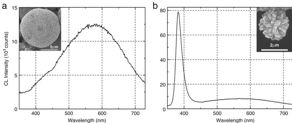
Fig. 6. Cathode luminescence (CL) spectra of the self-assembled one-dimensional ZnO nanorod-based: (a) microspheres, inset with the corresponding SEM image; and (b) radial spherical structures, inset with corresponding SEM image.
