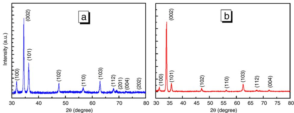
Fig. 1. XRD pattern of the ZnO nanorods: (a) microspheres; and (b) radial structures synthesized by the biopolymer-assisted self-assembly method. All diffraction peaks are indexed in agreement with the JCPDS 036-1451 card for ZnO.
