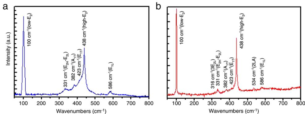
Fig. 5. Micro-Raman scattering spectra of the self-assembled ZnO nanorod-based: (a) microspheres; and (b) radial structures.
