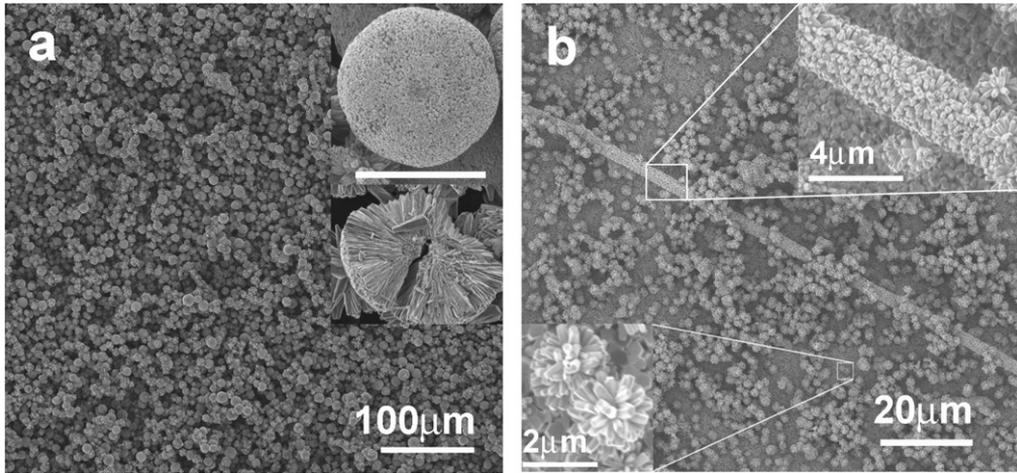
Fig. 2. Scanning electron micrographs of the ZnO architectures chemically grown by the biopolymer-assisted self-assembly method: (a) the overall morphology of ZnO nanorod-based microspheres. The insets are individual (up) and micromechanical broken microspheres (down), the scale bar in the inset is 10  $\mu\text{m}$ ; (b) ZnO radial architectures from one-dimensional ZnO nanorods and insets with magnified images.
