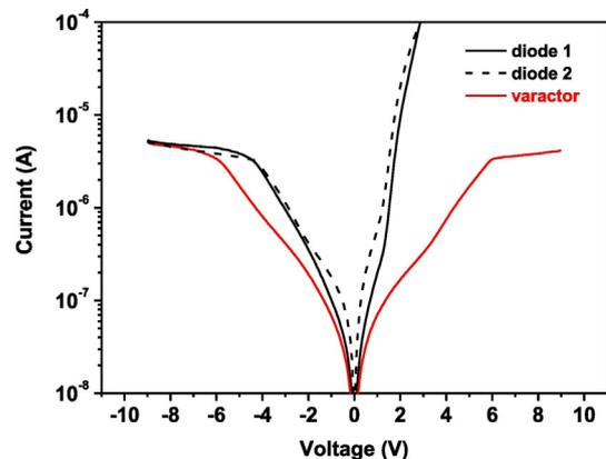
Fig. 6.  $I$ - $V$  curves of the single capacitors with a thin dielectric layer and the varactor formed by the capacitors.
