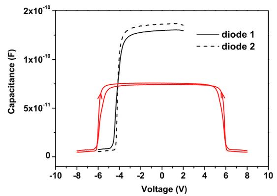
Fig. 8.  $C$ - $V$  curves of the MISH varactor measured for both voltage directions. Also shown are  $C$ - $V$  curves of the capacitors forming the varactor.
