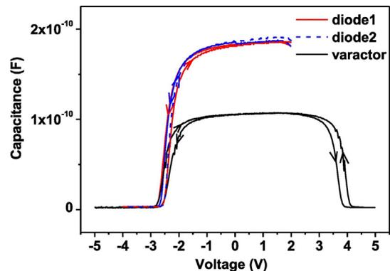
Fig. 3. *C-V* curves of single diodes of the varactor and the *C-V* curve of the varactor composed of the two diodes.
