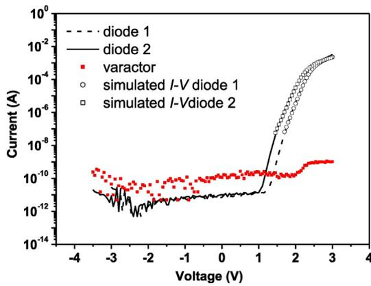
Fig. 4.  $I$ - $V$  curves of the single diodes of the varactor and a  $C$ - $V$  curve of the varactor composed of the two diodes.
