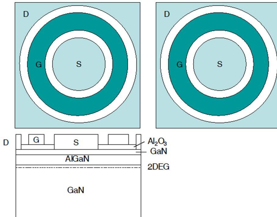
Fig. 1. View and the cross-section of the two Schottky gate capacitors forming the varactor. G is the Schottky gate and D is the Ohmic contact. Varactor is formed between the G electrodes.
