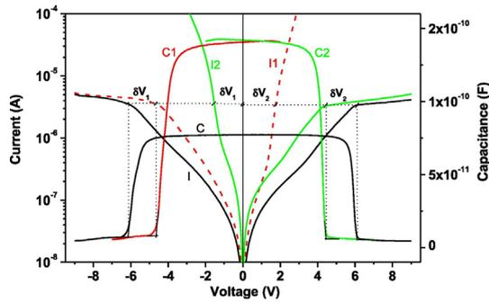
Fig. 7.  $I$ - $V$  and  $C$ - $V$  curves of the MSM varactor with the dielectric layer and voltage drops on the single capacitors compared with the differences between the transition voltage of the varactor and the threshold voltage of the single capacitors.
