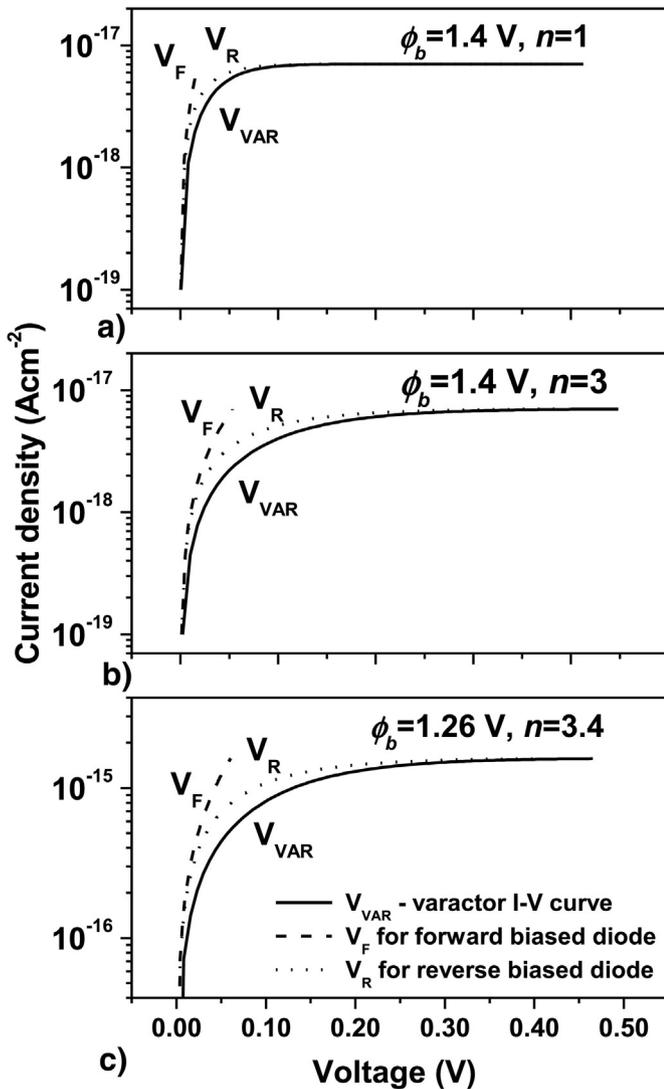
Fig. 2. *I-V* curve of a varactor with two back-to-back connected diodes and voltage drops on forward  $V_F$  and reverse  $V_R$  biased diodes for a) Schottky barrier height  $\phi = 1.4$  V and ideality factor  $n = 1$  and b)  $\phi = 1.4$  V and ideality factor  $n = 3$  and c)  $\phi = 1.26$  V and ideality factor  $n = 3.4$ .
