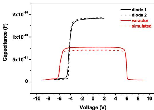
Fig. 5.  $C$ - $V$  curves of single diodes with a thin dielectric layer and the varactor formed by the capacitors. Also shown is the simulated  $C$ - $V$  curve of the varactor from the measured  $C$ - $V$  curves of the single capacitors.
