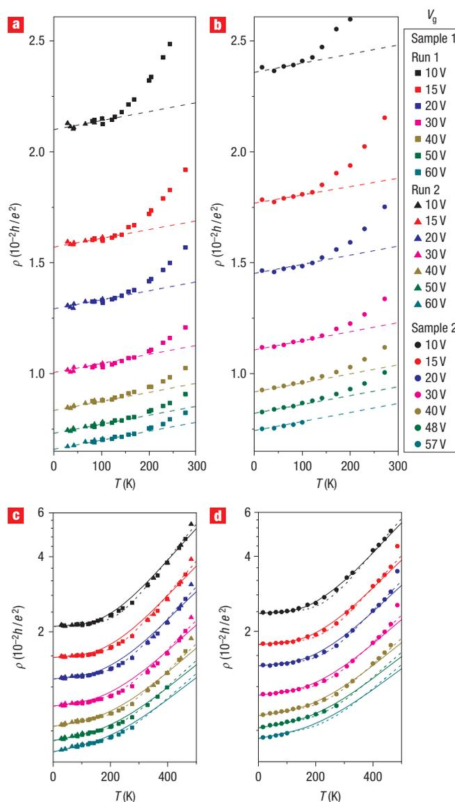
**Figure 1** Temperature-dependent resistivity of graphene on SiO<sub>2</sub>.
