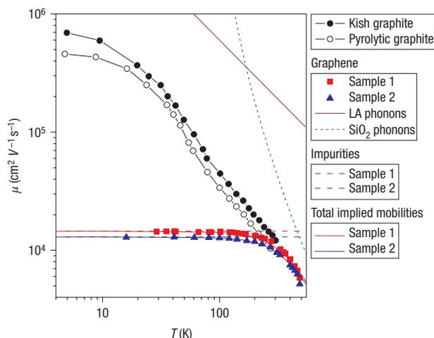
**Figure 3** Temperature dependence of mobility in graphene and graphite.
