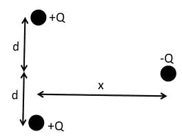
We have equal charges +Q distance 2d away from each other as shown in the figure below. A charge, -Q is brought in from infinite distance away to the position shown.
