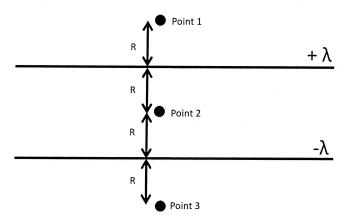
Find the direction and the magnitude of electric field at point 1,2, and 3
