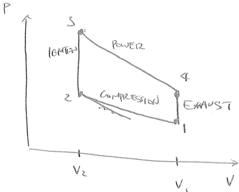
$$\eta = \frac{|Q_{23}| - |Q_{41}|}{|Q_{23}|} \quad \text{vs} \quad \frac{T_4 - T_1}{T_3 - T_2}$$
