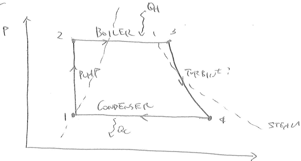
$$\eta = 1 - \frac{Q_C}{Q_H} \Rightarrow 1 - \frac{H_4 - H_1}{H_3 - H_2}$$
