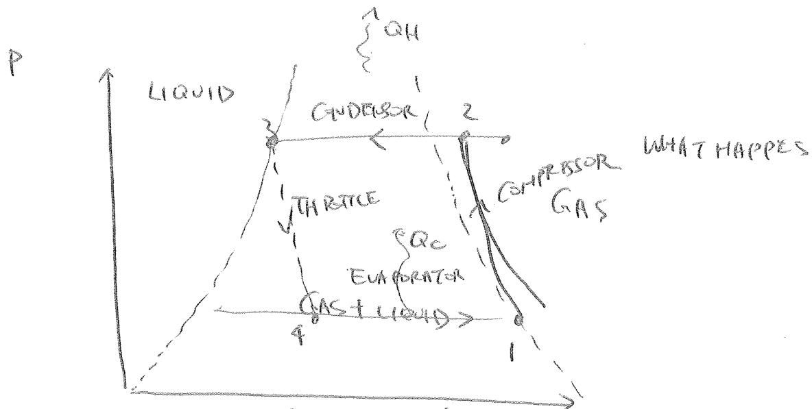
$$COP = \frac{Q_c}{Q_H - Q_c} = \frac{H_1 - H_4}{H_2 - H_3 - H_1 + H_4}$$
