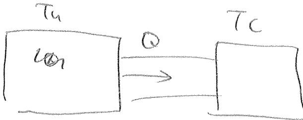
$$\begin{aligned}\Delta S_{\text{univ}} &= -\frac{Q}{T_H} + \frac{Q}{T_C} \\ &= Q \left( \frac{1}{T_C} - \frac{1}{T_H} \right) > 0\end{aligned}$$
