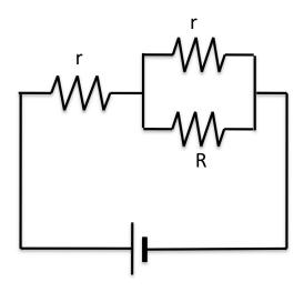
A battery with voltage V supplies current to the circuit shown below. There are three resistors: r is a constant resistor while R is a variable resistor.
