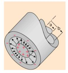
(a) Calculate the capacitance per unit length for the cylindrical capacitor as shown left. The inner space between the conductors is vacuum.
