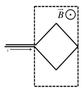
Calculate the force if the metal square has been inserted further into the magnetic field. Everything else remains the same. The square has sides of 1 m, the magnetic field is 0.1 T, and the current is 1 A. Magnetic field is only present in the dotted square as indicated in the figure.
