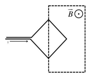
Calculate the force due to magnetic field on a wire which has been shaped into a square shape as shown left. The square has sides of 1 m, the magnetic field is 0.1 T, and the current is 1 A. Magnetic field is only present in the dotted square as indicated in the figure.
