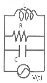
Find the complex impedance for the parallel RLC circuit as shown. Assume that we have a voltage source for which we can adjust the angular frequency  $\omega$ .  $V(t)=V_{max}cos(\omega t)$ .
