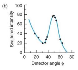
The strongly directional scattering could only be explained by assuming diffraction of an incident wave, with wavelength  $\lambda = h / p$ , where p was the momentum of the electrons
