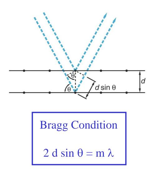
X-rays are diffracted by the periodically arranged atoms in a crystalline lattice
