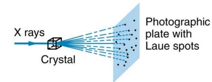
X-rays are diffracted by the periodically arranged atoms in a crystalline lattice
