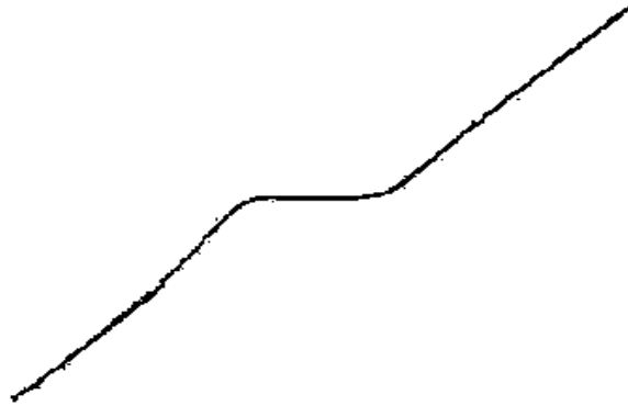
Figure 14: Typical Mr. SQUID ® V-I characteristic. Compare with Fig. 6. The central region has low resistance because the current is less than the Josephson junctions' critical current there. For currents greater than the critical current, the SQUID is Ohmic, with a normal state resistance given by the slope.
