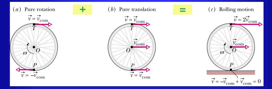
The motion of any round body rolling smoothly over a surface can be separated into purely rotational and purely translational motions.
