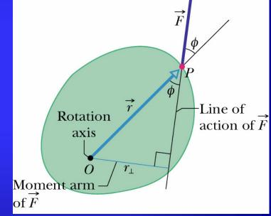
Sign: Torque >0 if body rotates counterclockwise. Torque <0 if clockwise rotation.
