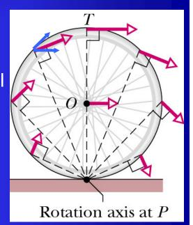
A rolling object has two types of kinetic energy  $\rightarrow$  Rotational: 0.5  $I_{COM}\omega^2$  (about its COM).
