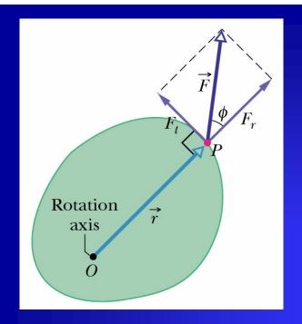
Radial component, F<sub>r</sub>: does not cause rotation → pulling a door parallel to door's plane.
