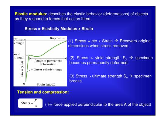
$$Strain = \frac{\Delta L}{L} \qquad (\text{ fractional change in length of the specimen})$$
