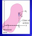
Each force  $F_{gi}$  produces a torque  $\tau_i$  on the element of mass about the origin O, with moment arm  $x_i$ .
