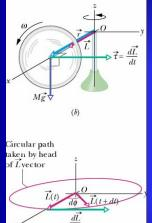
If released with shaft's angle slightly upward  $\rightarrow$  first rotates downward, then spins horizontally about vertical axis  $z \rightarrow$  precession due to non-zero initial angular momentum
