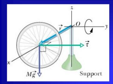
Gyroscope: wheel fixed to shaft and free to spin about shaft's axis.
