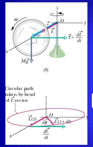
If released with shaft's angle slightly upward  $\rightarrow$  first rotates downward, then spins horizontally about vertical axis  $z \rightarrow$  precession due to non-zero initial angular momentum
