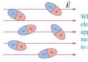
When an electric field is applied, the molecules tend to align with it.
