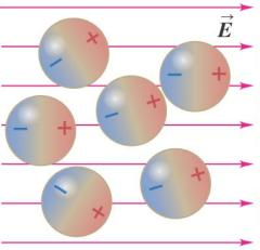
An electric field causes the molecules' positive and negative charges to separate slightly, making the molecule effectively polar.
