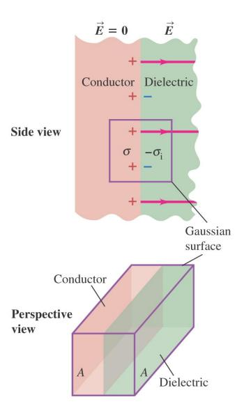
Flux through Gaussian surface (enclosed free charge /  $\epsilon_0$ )
