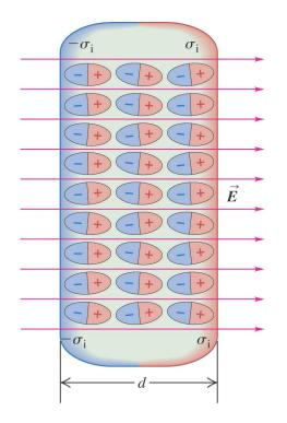
Polarization of a dielectric in electric field gives rise to bound charges on the surfaces, creating  $\sigma_i$ , -  $\sigma_i$ .
